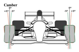
**Positive Camber**: If the top of the tire leans outward, away from the car's center, the tire has a positive camber angle.
