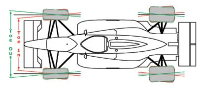
Toe in is a comparison of the distance between the front of the tires and the rear of the tires. If the two tires are parallel, the two distances are the same; toe is zero. If the distance is smaller in the front of the tires than the rear, the difference is equal to the amount of toe-in. If the distance is larger in the front of the tires than the rear, the difference is equal to the toe-out.
