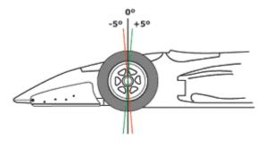
Caster is a directional control angle that helps the driver keep the front tires straight down the road and return the steering straight ahead after turning a corner.
